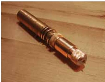
Figure 7. This is the die cutting device fabricated to fit in the routers ½-in. collet along with a compression added to allow for exact pressure to be applied during cutting.
